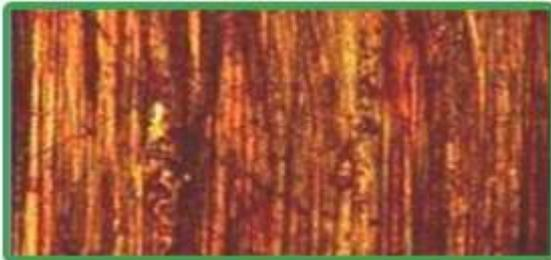
Fig. 11 : Wear screen of the test panel (Zoom x100) , Test load 1,000 N, 65,000m
